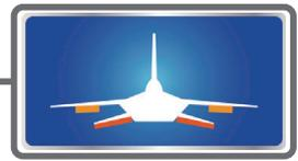
This mixing is used to correct changes (elevator direction) generated when the camber flaps (speed flaps) are used.
