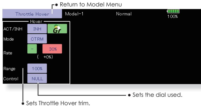
The Throttle Hover function trims the throttle near the hovering point. Normally, use it with hovering conditions. Changes in rotor speed accompanying changes in the temperature, humidity, and other flight conditions can be trimmed. Adjust the throttle so that rotor rotation is most stable. More delicate trimming is also possible by using this function along with the Hover Pitch function.
