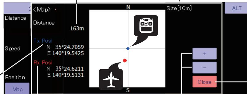
●It is the size of the map. It is the distance from the Tx position (reference point at the center of the map) to the end. Change the size with the +/- button.
