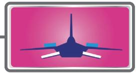
This mixing is used when you want to mix the elevators with airbrake (spoiler) operation. It raises the elevators to correct for drooping of the nose during airbrake operation.
