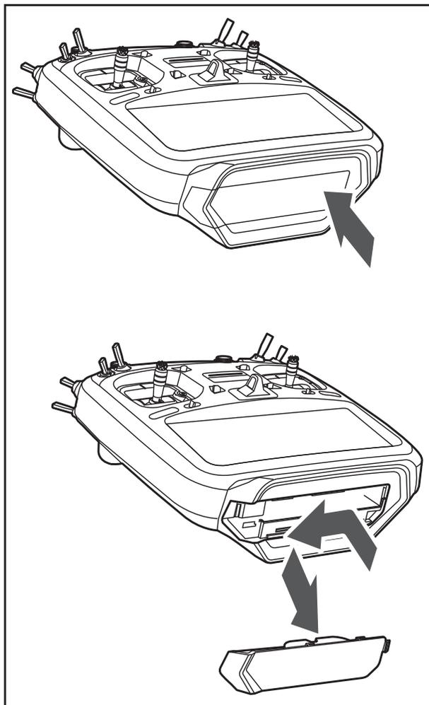
2. Pull out the Battery removal clip and slide out the battery.
