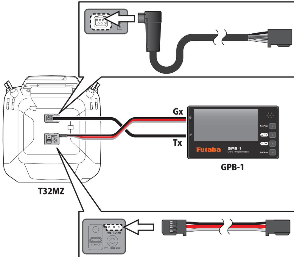
Connect the T32MZ's **"S.I/F"** (S.BUS) connector to the GPB-1's **"Gx"** connector with the **CGY760R Connection Cable** supplied with the GPB-1.
