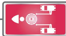
This function is dedicated mixing used in needle adjustment of an engine that uses a fuel mixture control carburetor.
