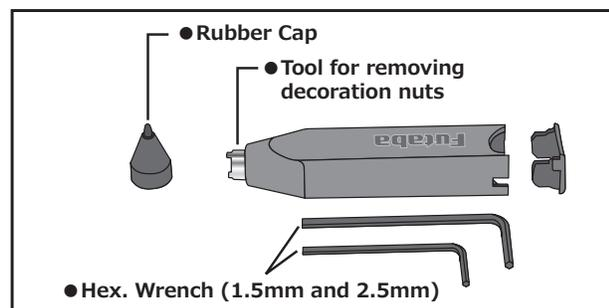
A special toolbox is included with your T32MZ. This allows you to make all of the mechanical adjustments that may be needed.
