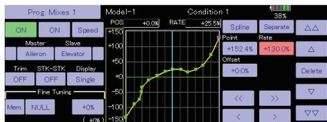
Changed to line or spline mode, the curve is retrieved as 17 points curve.
