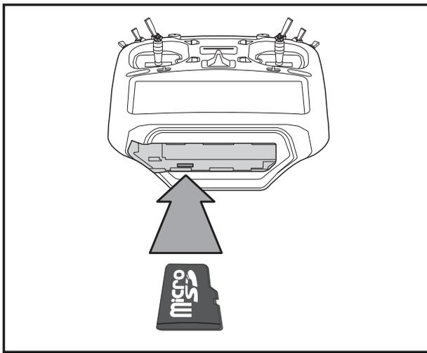
1. Insert the microSD card containing the update file into the card slot.
