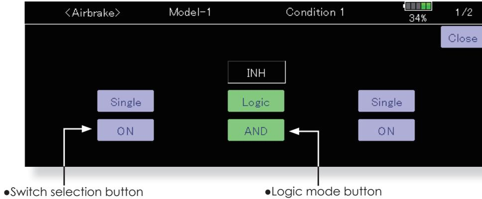
1. The logic selection dialogue appears when you push the logic mode button. The 3 types of logic, either AND, OR or EX-OR, can be selected.
