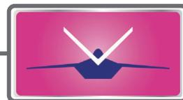
This function let's you adjust for left and right rudder angle changes at elevator and rudder operation of a V-tail airplane.
