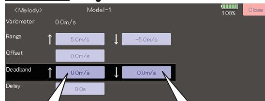
When the variometer is less than this value, Vario melody is not output.
