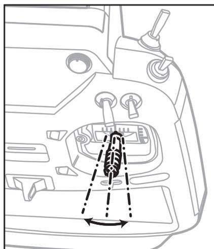
Use the attached 1.5 mm hexagonal wrench (inside stylus) to turn the screw clockwise to adjust the stick outwards, or counter-clockwise to tilt it inward.
