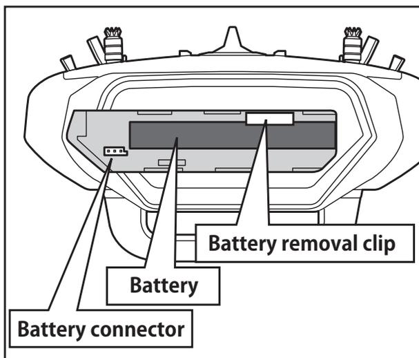
4. Connect the battery wiring as shown in the figure.
