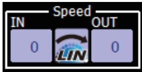
The speed during operation (including flight condition switching) can be adjusted. The servos operate smoothly at a constant speed corresponding to the speed set for them. The operation speed (In Speed) and the return speed (Out Speed) can be set individually.
