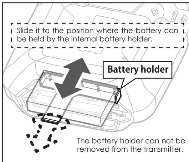
3. Remove the battery from the battery holder.
